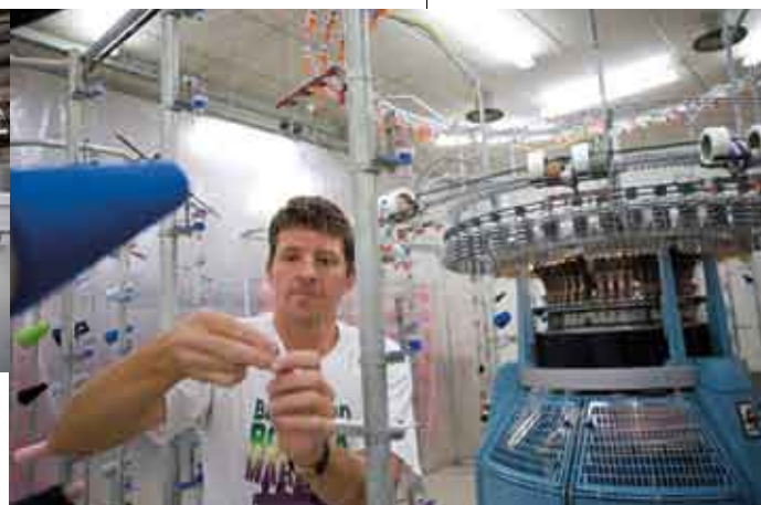
Maurice Brown, Knitting Supervisor, sets up a striper knitting machine
