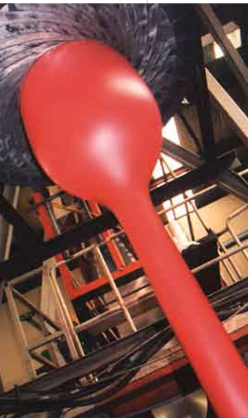
HDPE bubble being blown during the extrusion process at Elldex's Albany plant
